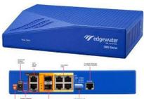
Edgewater Networks' EdgeMarc 2900e Intelligent Edge is ideally suited for Hosted PBX or SIP Trunking applications that do not require analog lines. The solution supports bi-directional data rates up to 1Gbps and up to 300 concurrent calls.
